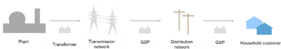
Figure 7: Overview of where losses can occur during electricity delivery to the user
